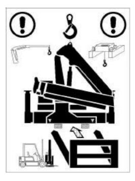
4. During the transport by land and sea, fix the crane or its container to the means of transport (body, container, hold, etc.).
