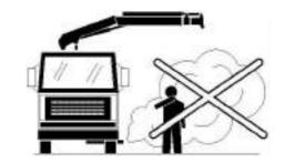
If the operator is exposed to exhaust fumes move the exhaust pipe outlet point further away from the operating position (e.g. using removable flexible hosing).
