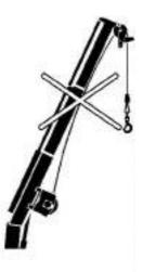
In the event of broken or permanently deformed strands on the rope (caused by crushing, excessive strain, etc.) contact an authorised assistance centre for immediate substitution of the rope.
