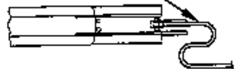
Secondary boom overhoist prevention device electrical cable
