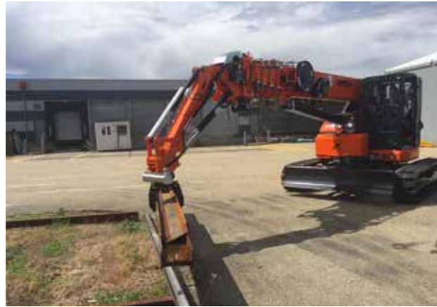
Grabber manipulator JIB303GR on SPK60, FRANCE
