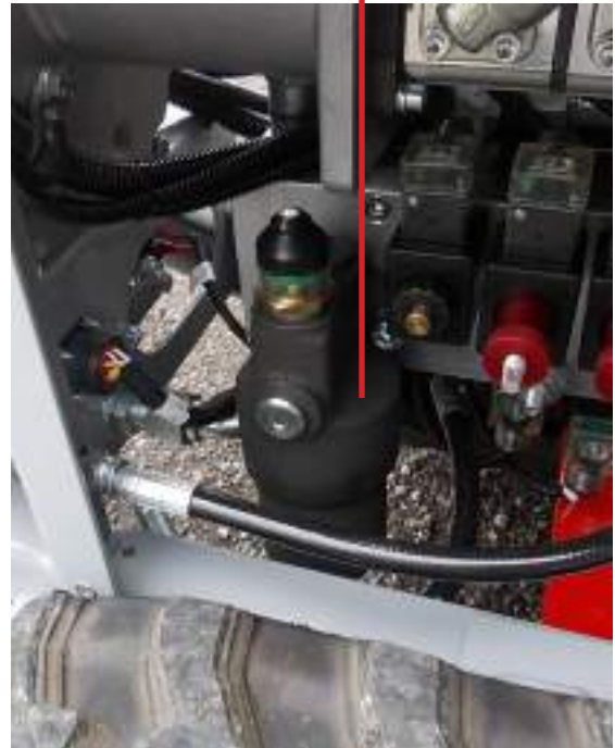
DELIVERY LINE HYDRAULIC OIL FILTER
