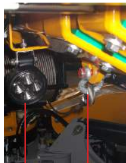
HOOK FOR SETTING ROPE ASIDE (NO LIFTING!)
