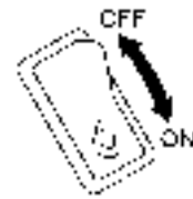
Main winch switch
