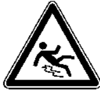
Warning of danger through slipping
