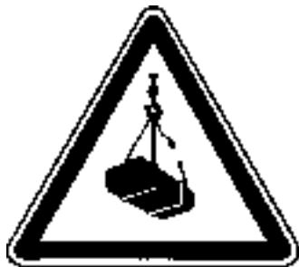
Warning of hanging load
