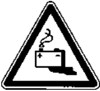
Warning of danger through batteries
