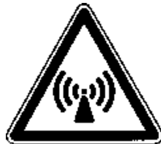
Warning of electro-magnetic field
