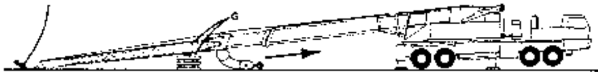
Fig. 4-9 Fly Section Removal
