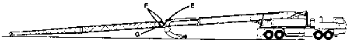
Fig. 4-12 Attaching The Jib
