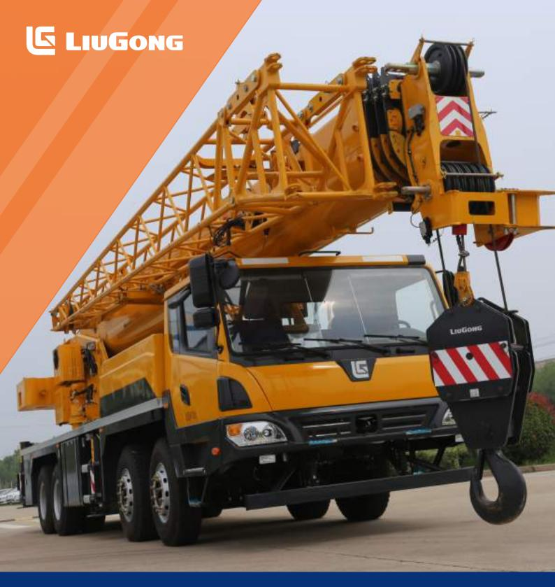
Main Boom45 mJib16 mMax Boom Length (Main Boom+Jib)61 mMax Lifting Capacity55 TCounterweight4.5T fixed + 4T fixable
