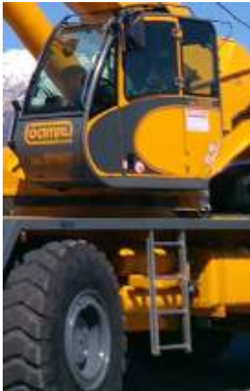
Cabin access ladder (left side)
