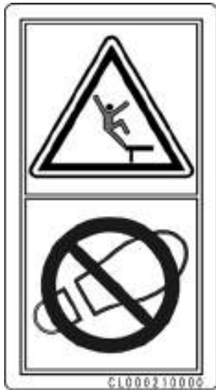
(23) Cautions on the fenders (CL000210000)
