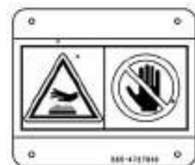
(37) Cautions against the risk of burns in the engine room (585-4727600)
