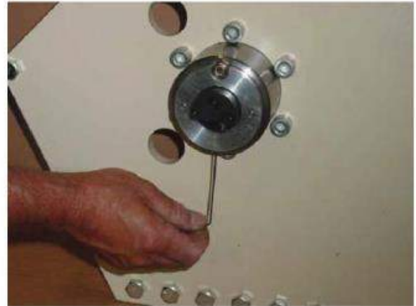
Figure 4: Loosen set screw on unit flange.
