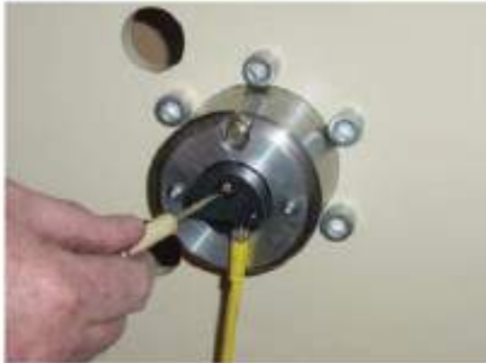
Figure 8: Remove LLI (Last Layer Indicator) programming screw.
