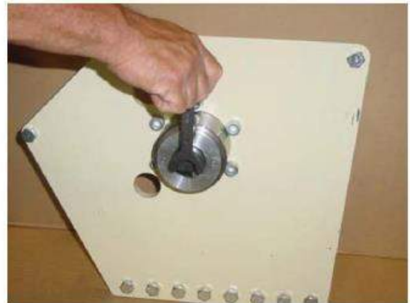
Figure 6: Tighten set screw.
