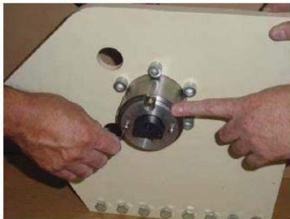
Figure 3: Secure with two screws.
