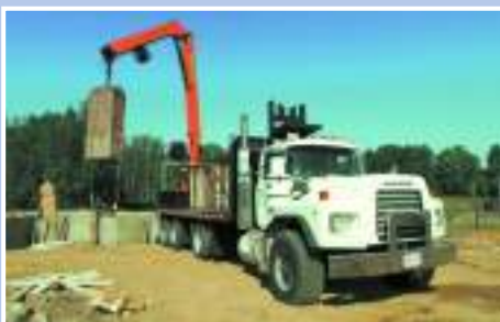
The PW series of cranes can be front or rear mounted on almost any 3 or 4 axle truck
