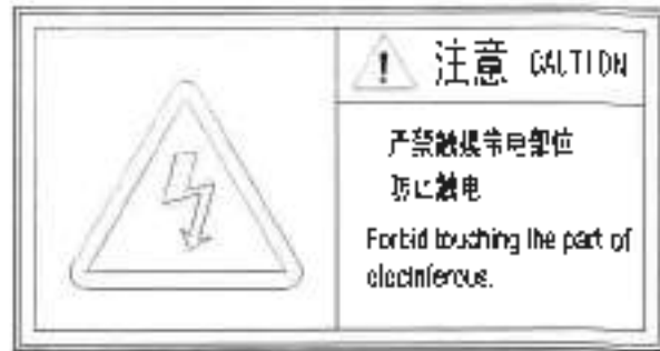
Fig.2-26 Caution Label for electric shock
