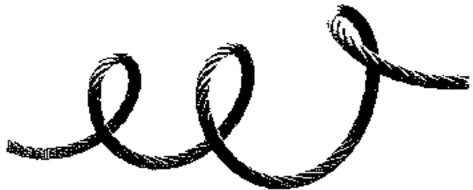
Figure 39. A corkscrewed rope; the condition came about as a result of the rope being pulled around an object having a small diameter.
