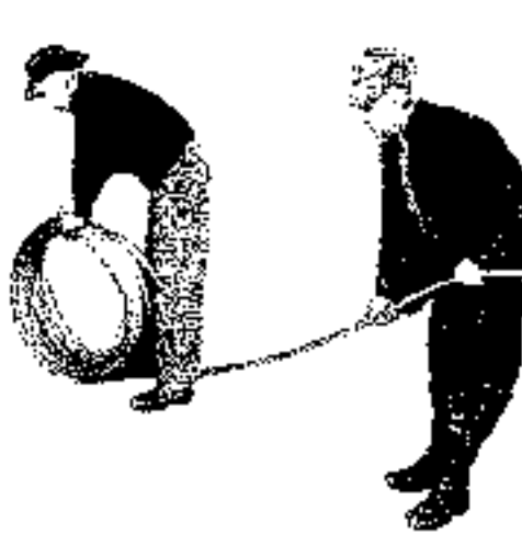
Figure 16. Perhaps the most common and easiest uncoiling method is to hold one end of the rope while the coil is rolled along the ground.
