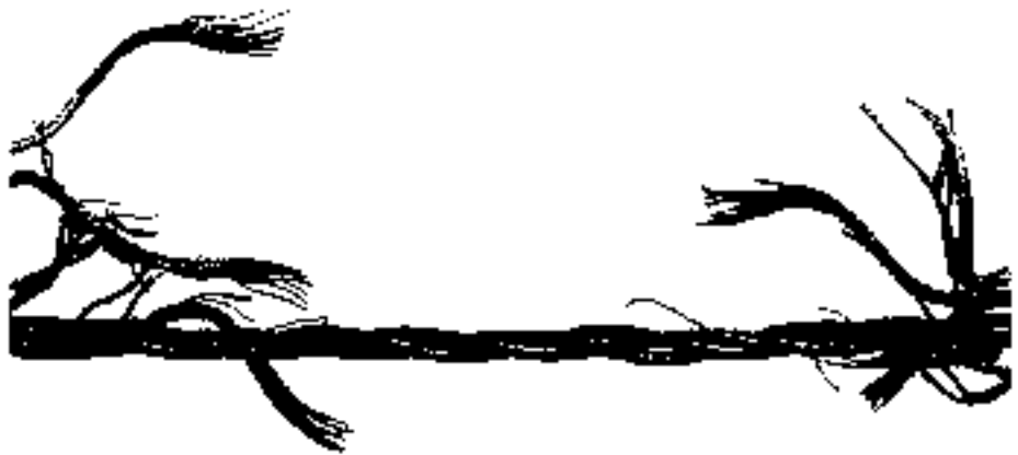
Figure 52. This is the appearance of a typical tension break, a result of overloading.
