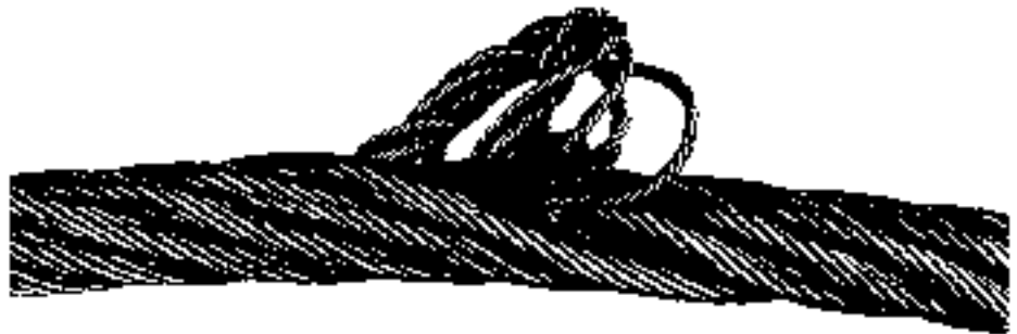
Figure 48. An occurrence that is called a pop and core
