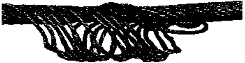
Figure 49. This is a typical bird cage condition.
