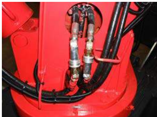
Illustration 5 showing crane ready for emergency winching
