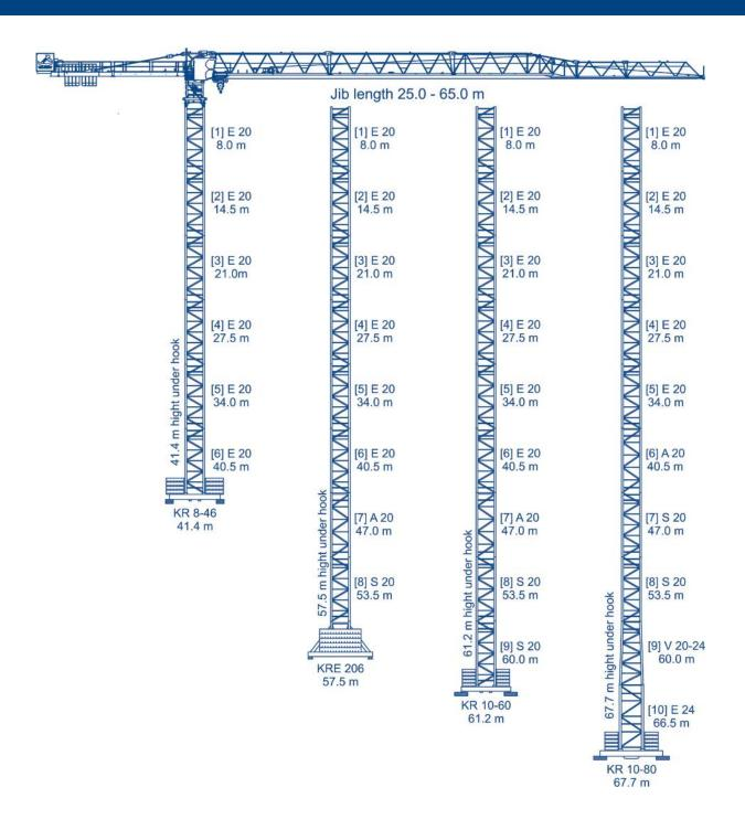
Tower combinations according to C 25 wind data.
