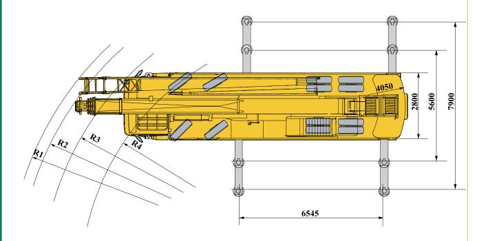
The medium and large tonnage products increase the full-scale shape and size parameter map, and the corresponding weight tail radius of gyration A: Approach angle B: Departure angle C: plane height on the frame D: vehicle height E: vehicle width R1: minimum turning radius of the arm head (the main arm and the jib are determined according to the size) R2: Minimum turning radius of the body R3: minimum turning radius H: minimum ground clearance.
