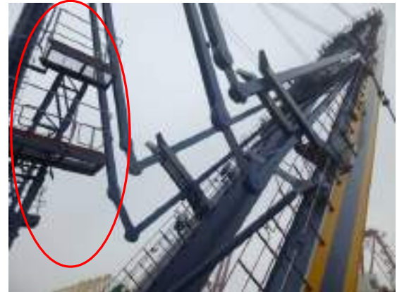
Figure 1-473: Maintenance Platform for Boom Forestays
