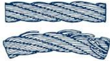
Figure 4-16: Detecting wire breaks by bending the rope
