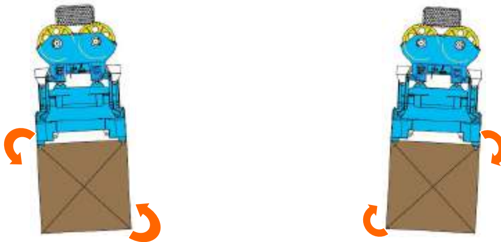
Figure 1-11 Spreader Forward List ↖ and Backward List ↗
