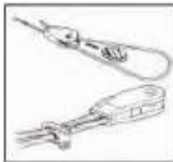
Figure 1-34 Becket and Wedge
