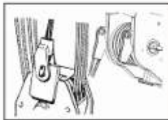
Figure 1-26 Main Hook and Nipple
