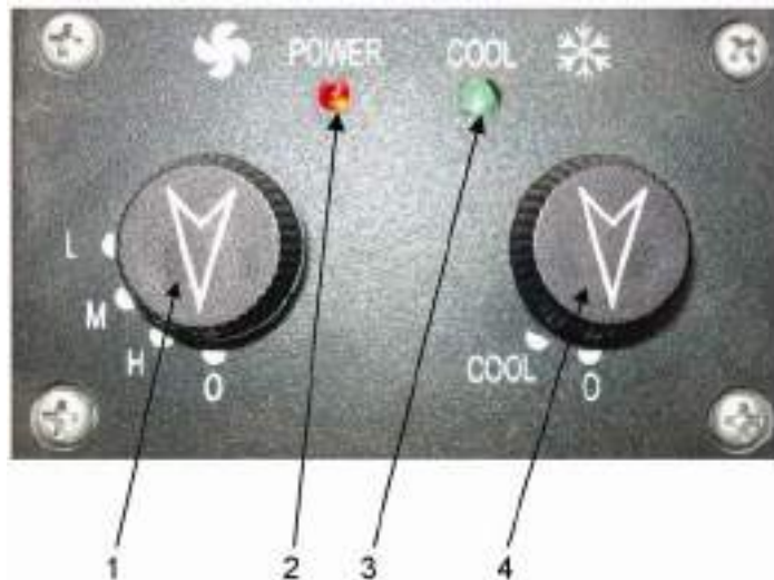
Figure 06 – 4 Air Conditioner Control Panel
