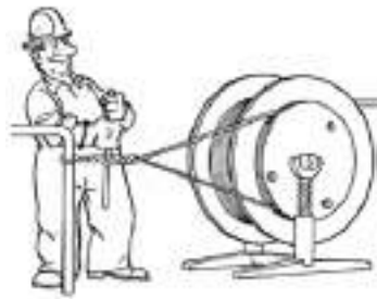
(a) Brake the wire flange with the brake plate on the winding shaft
