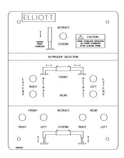
**NOTE**: When deploying outriggers, always set the beams to either full or mid-span prior to lowering outrigger jacks. Always be sure to use correct load chart based on outrigger span. When stowing/raising outriggers, always raise outrigger jacks prior to retracting beams. Always set center front stabilizer last and retract first when stowing.
