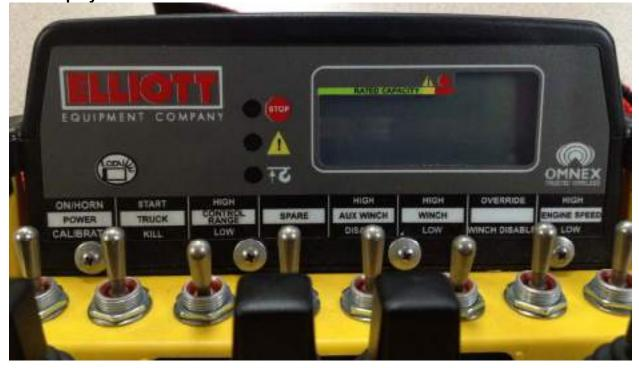
Elliott remote controls provide the operator with the same load and capacity information to the operator using the remote controls as if they were operating from the operator's cap or platform. This provides the operator in the platform or at the hook point with boom length, angle and load radius information along with allowable load and actual load values
