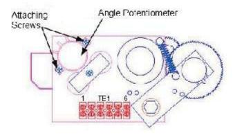
Image 15 Zeroing the Angle Sensor
