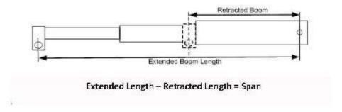
Image 13 Extended Length - Retracted Length = Span
