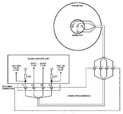
Image 26 Swing Sensor Schematic
