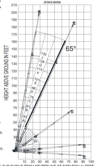
NOTE: 1. Operate jib by radius when main boom is fully extended.
