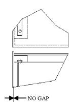
Properly aligned and adjusted wear pad. The holes in the retainer plate are concentric with the threaded holes in the smaller boom section and the wear pad is tight against the side plate of the larger boom section. When wear pads are properly aligned and adjusted, install capscrew and torque to 75 ft-lb (100N.m)
