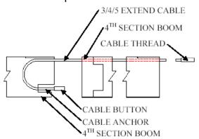
install keeper plate and capscrews, keeper plate will lock both the extend and retract cables in place. Coil 5/4/3 retract cables temporarily into 5<sup>th</sup> section.
