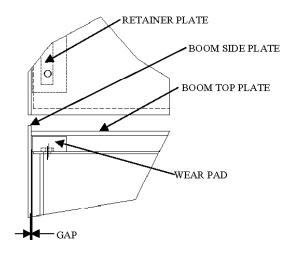
**Needs adjustment.** The capscrews can not be installed and there is a gap between the wear pad and side plate of the larger boom section
