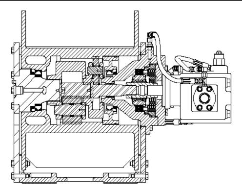
The planetary hoist is designed to utilize a geroler, gear, or piston motor, driving through a multipledisc oil brake, through a pair of planetary gearsets to the cable drum.
