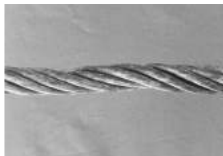
Local reduction of rope diameter
