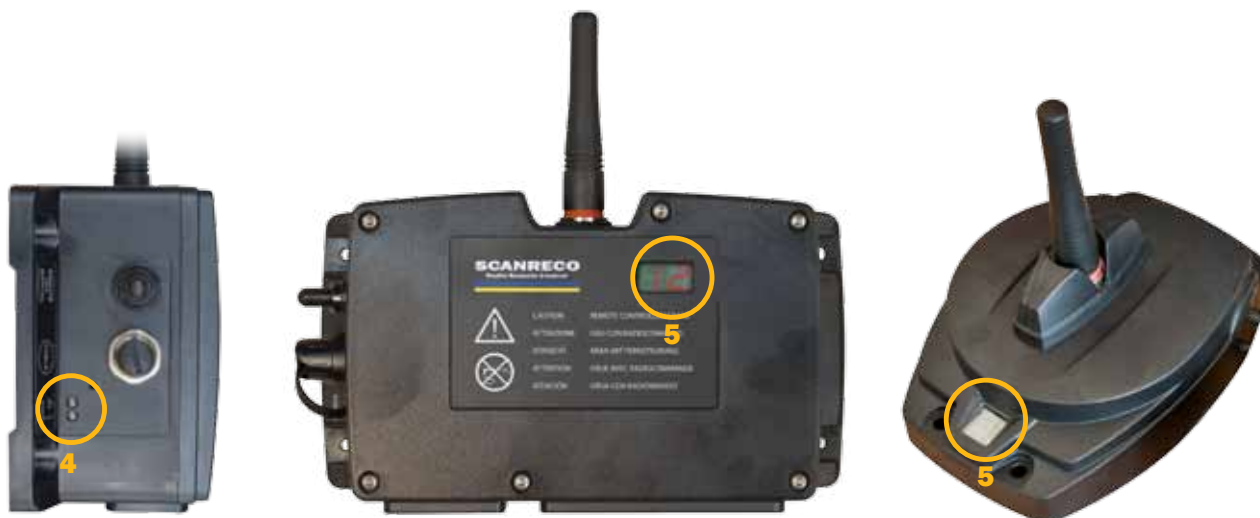
Position 4: Status LEDs
