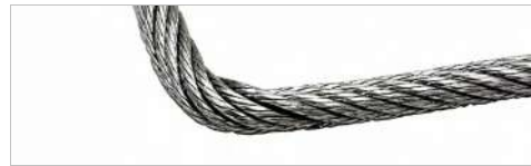
There is a kink in the wire rope. This results from violent external forces being applied to the wire rope.
