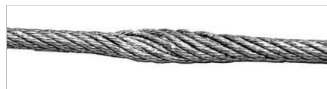
The wire rope is flattened at one point. This results from the wire rope being pinched.
