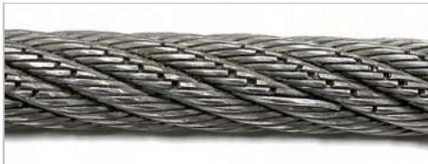
Multiple broken wires. Broken wires are signs of normal wear of the wire rope. They occur when the wire rope is bent on the reels under load.
