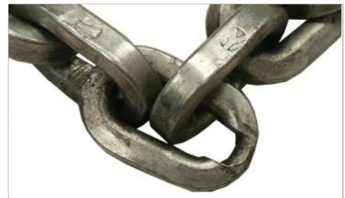
The chain link is heavily worn.
