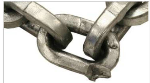
The chain link is mechanically damaged.
