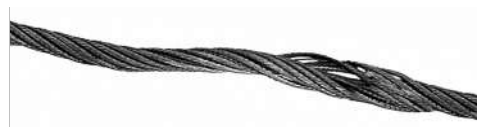
A bird cage has formed in the wire rope. This results from violent untwisting of the wire rope.
