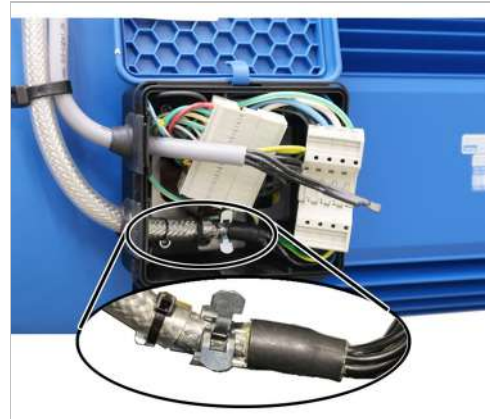
Screening clamp connection in connector housing
