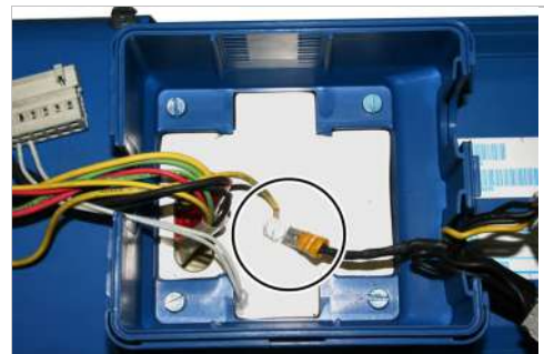
Cable lug in connector housing
