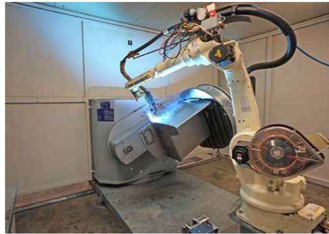
The structural steel construction of the trolley frames is carried out with the aid of a welding robot. This ensures short throughput times and consistent welding performance.
