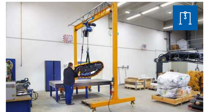
Lightweight mobile gantry LPK
