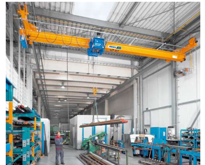
Type E monorail hoist on a type EDL underhung overhead travelling crane
