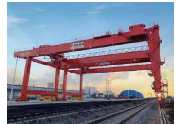
象屿集团轨道式集装箱门式起重机 Rail Mounted Container Gantry Crane for Xiangyu Group
